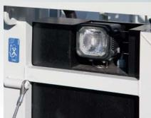
**230V halogen floodlights** on the sides and at the bottom of the rescue cage provide optimal lighting at the scene of operation.
